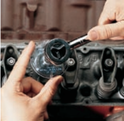
The Fel-Pro Torque-to-Angle Indicator eliminates uncertainty when torquing T-T-Y head bolts.
